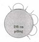
Recommended Attachments Through both tabs every 3 to 4 inches; (a) 1" to 1.5" Stainless steel #8 or #10 oval or flat head **Phillips** screws with Stainless finishing washers, (b) 1" to 1.5" Stainless steel pneumatic staples, or (c) 1.5" to 2" large-headed Stainless or aluminum nails. (Because Galvanized "roofing" nails will rust and "bleed" onto the dock bumper, they are not recommended.)
