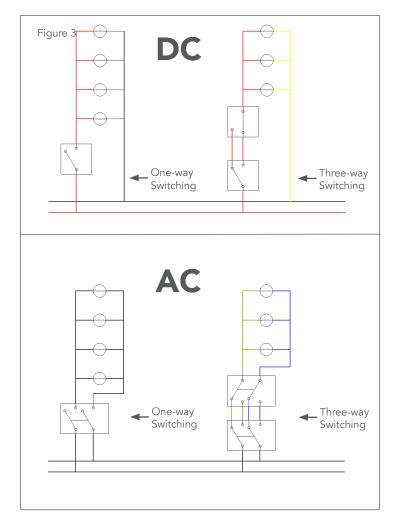
Many DC fixtures are polarity sensitive. These fixtures are typically provided with color coded wires. Please refer to **Table 1** to identify wiring based on its color. If the fixture is supplied with two white wires, it is not polarity sensitive.
